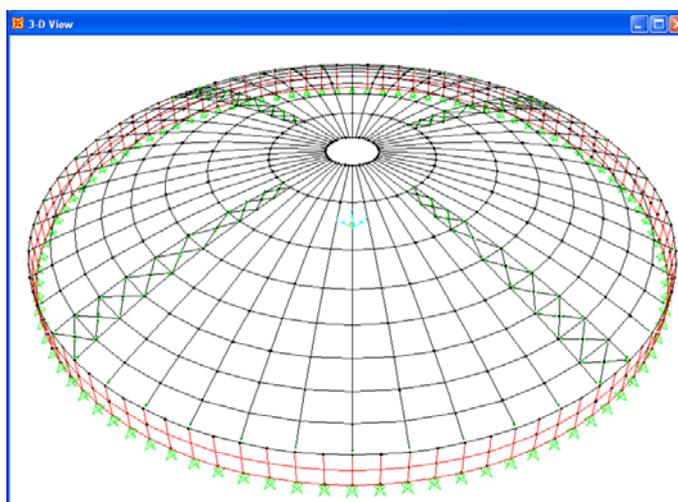
Fig. 1. Spatial researching model of the roof.
