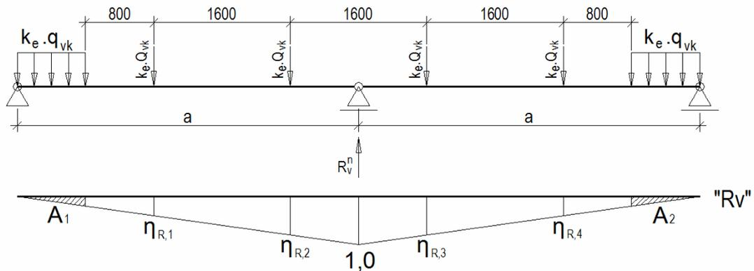
**Fig. 4.** Line of influence for support's reaction  $R_v^n$
