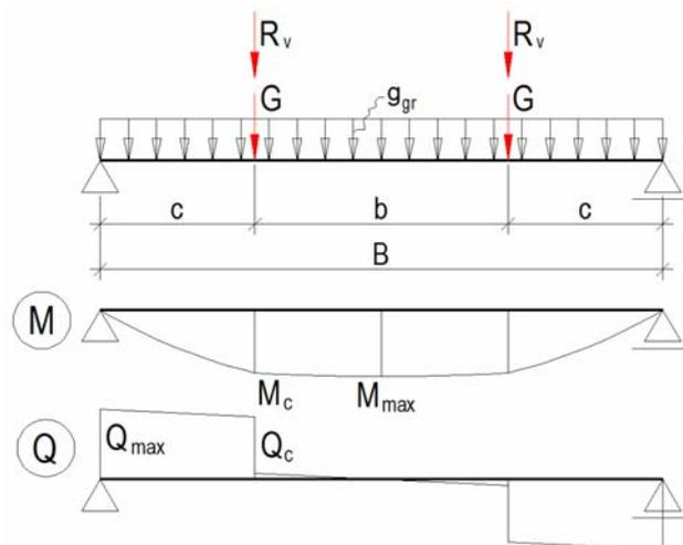
**Fig. 5.** Vertical loads on transverse beam and internal forces in it
