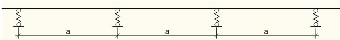
**Fig. 1.** Statical scheme of longitudinal beam for vertical moving loads.
