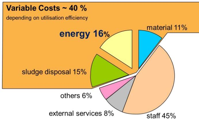
**Fig. 1. Analysis of operational costs for WWTP (≥ 50,000 PE) in Austria (LINDTNER)**
