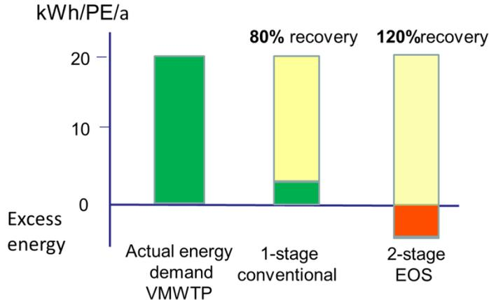
Fig. 5. Energy demand for actual situation, for a 1-stage activated sludge plant and for the 2-stage plant. In both cases the same situation was assumed, e.g.  $N/COD = 0,1$  in the influent, sludge digestion and same efficiency of aeration system, gas motors and generators
