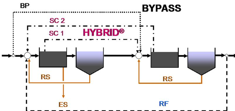
Fig. 3. Process scheme of the VMWWTP 2 – stage activate sludge treatment process
