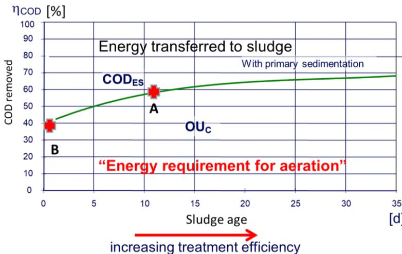
Fig. 1. COD balance for biological treatment by activated sludge process (ASP)
