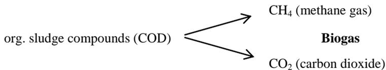
Sludge digestion converts part of the high entropy energy contained in the raw sludge to biogas which can be converted to low entropy electric and thermal energy:
