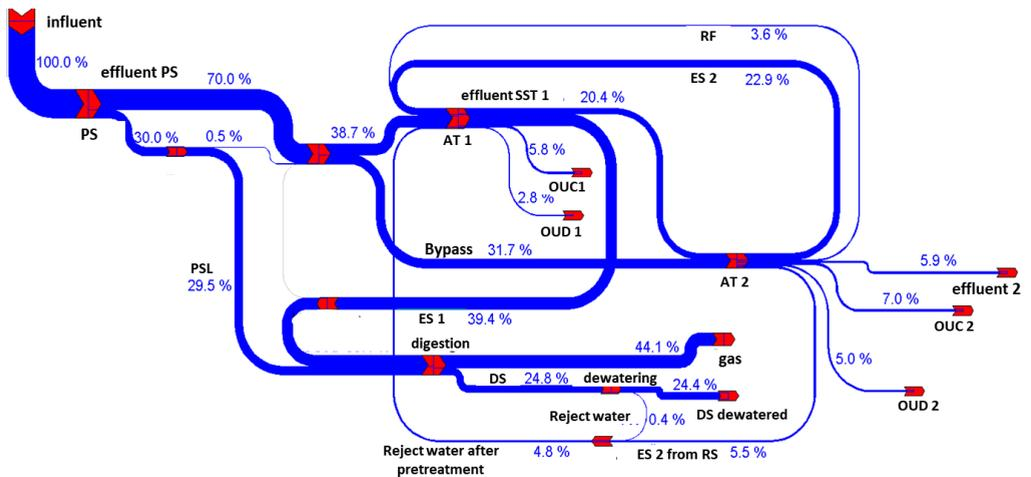
Fig. 4. Sankey diagram of mean yearly COD flow under design load (Kroiss, Svardal 2015)
