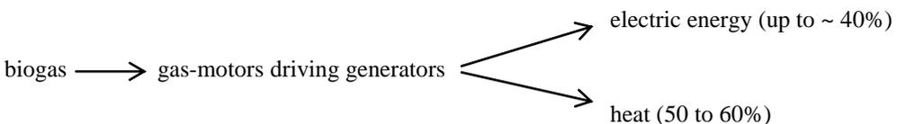
The electric energy generated can be either fed to the electrical grid or directly used as power supply of the treatment plant. The heat is normally used for heating the raw sludge to 35 to 40 °C (mesophilic conditions) and heating.
