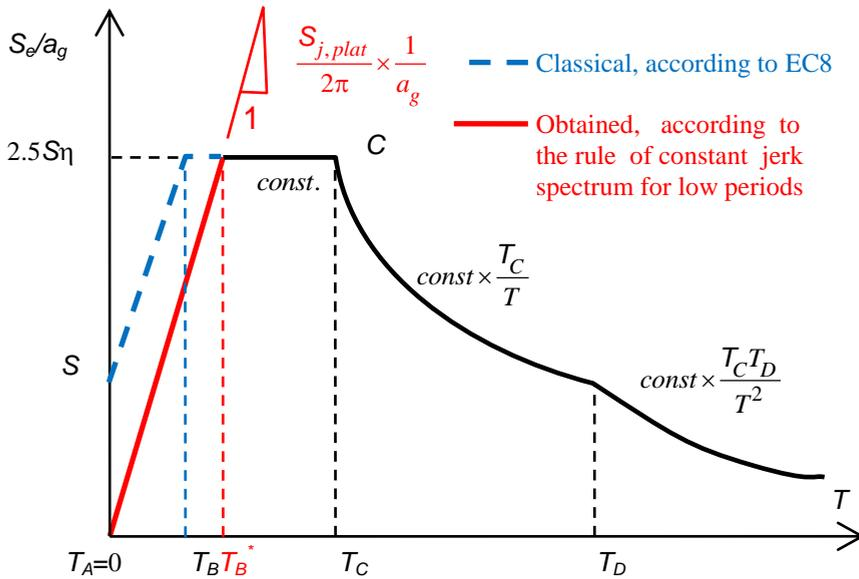
Figure 3. Elastic horizontal ground acceleration response spectra
