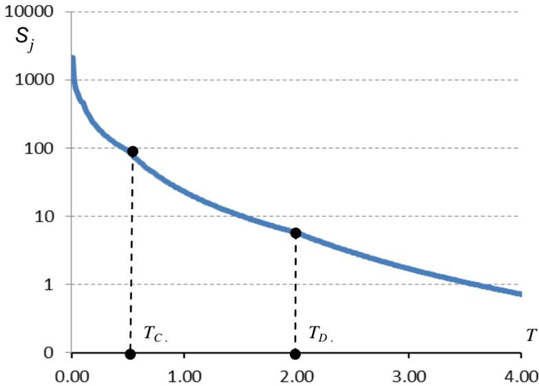
Figure 2. Elastic horizontal jerk response spectrum  $S_j$  according to (8), in log scale
