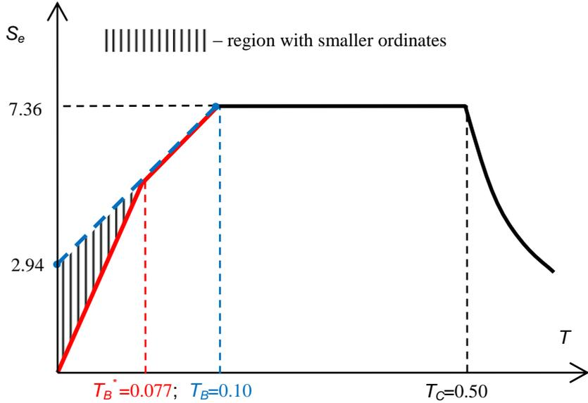
**Figure 5. Modified elastic horizontal ground acceleration response spectrum**
