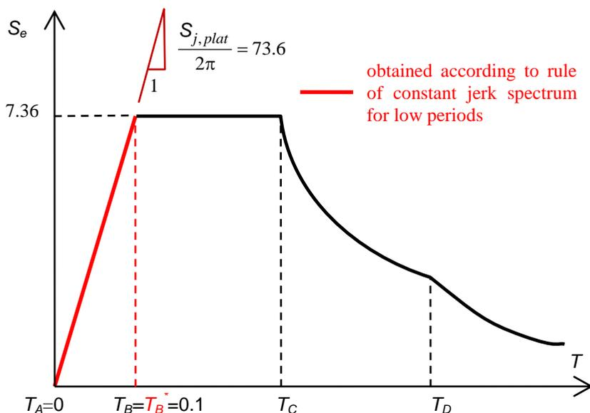
Figure 6. Modified elastic horizontal ground acceleration response spectrum in case of constant jerk for  $T \leq T_B$
