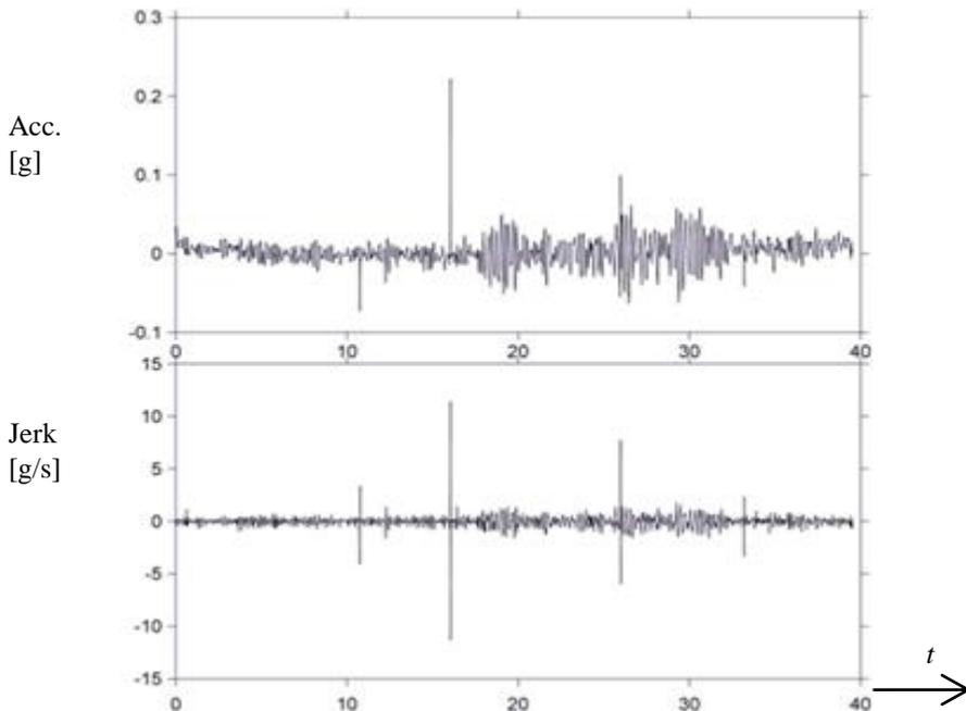
**Figure 1. Horizontal component of the recordings of the 1978 Tabas earthquake in Iran [4]**
