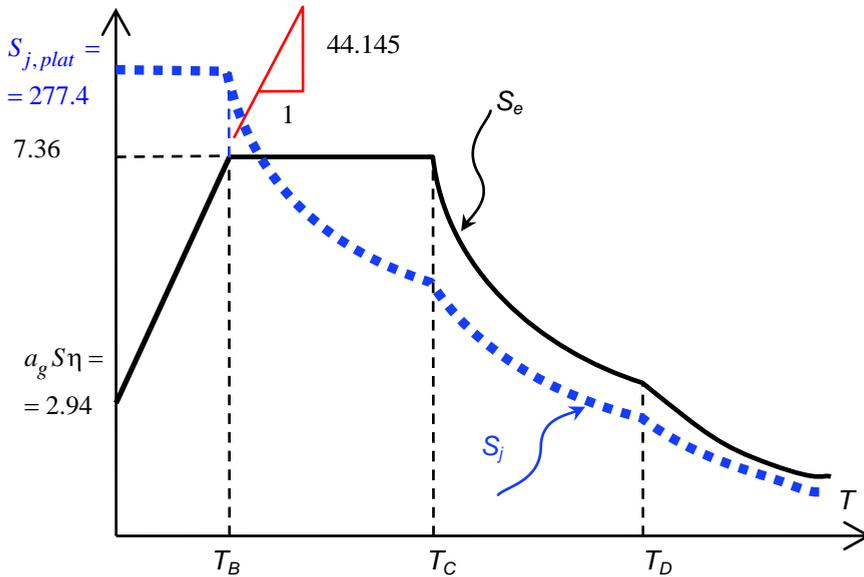
**Figure 7. Acceleration and Jerk response spectra according to modified relation between them (14), with example values, based on BG Annex**
