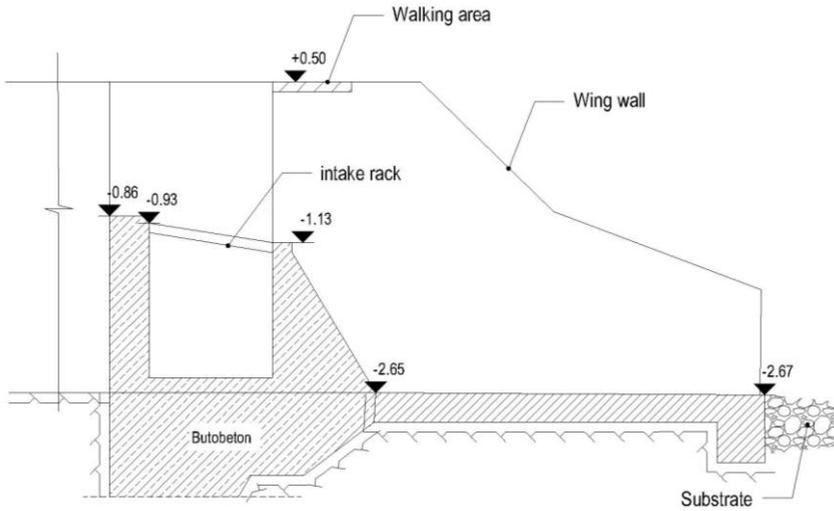
**Figure 5. Tyrolean intake with inlet rack in the weir – section**
