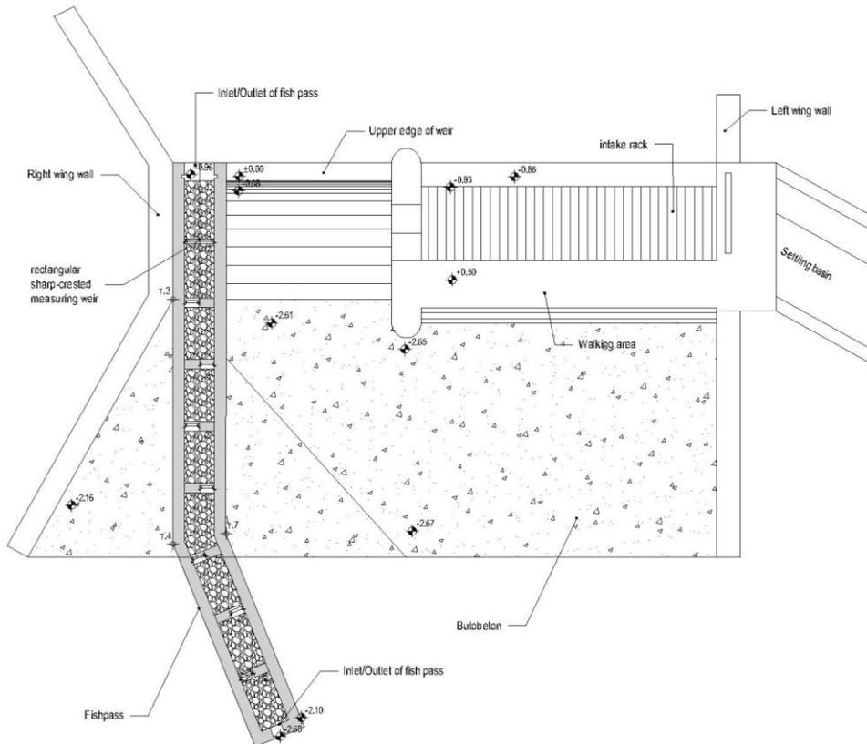
Figure 4. Pool pass with surface notches at Tyrolean intake with massive weir – layout
