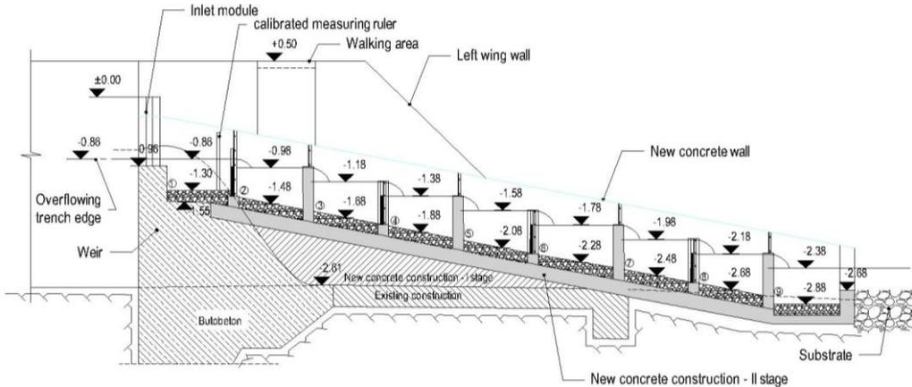
**Figure 6. Pool pass with surface notches at the walls between the pools – longitudinal section**
