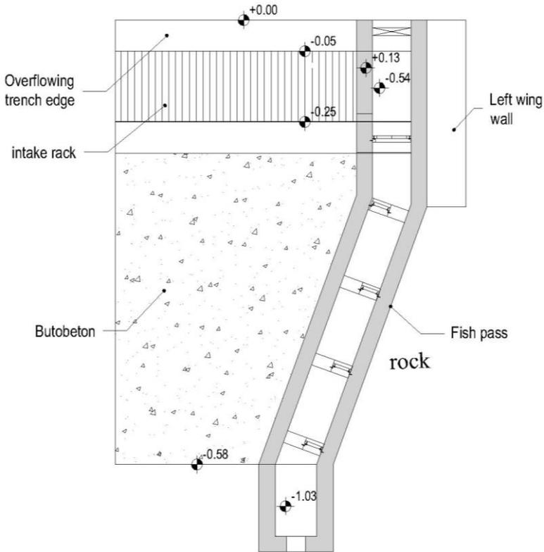
**Figure 2. Pool pass with surface notches at the walls between the pools – layout**
