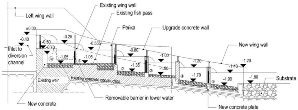
**Figure 9. The newly designed pool pass – longitudinal section**
