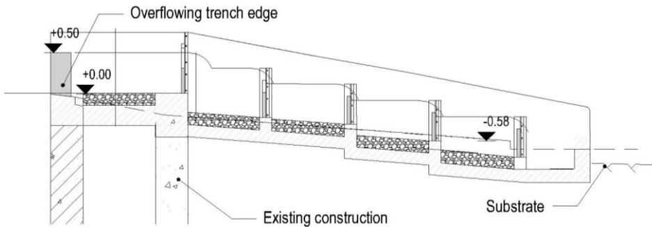
**Figure 3. Pool pass with surface notches at the walls between the pools – longitudinal section**
