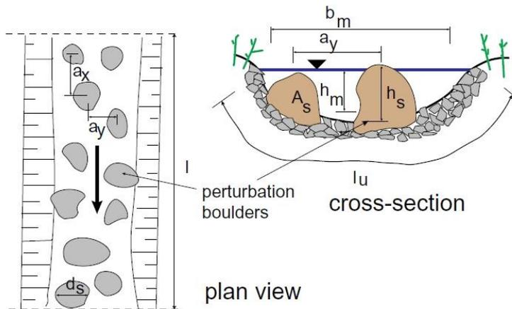
Figure 1. Typical solution of the bypass channel with perturbation boulders [2]
