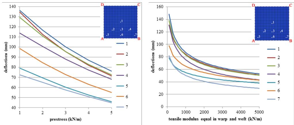
**Figure 7. Relation between membrane deflections, 7 different positions of the point load and membrane prestress (left) or tensile modulus (right)**
