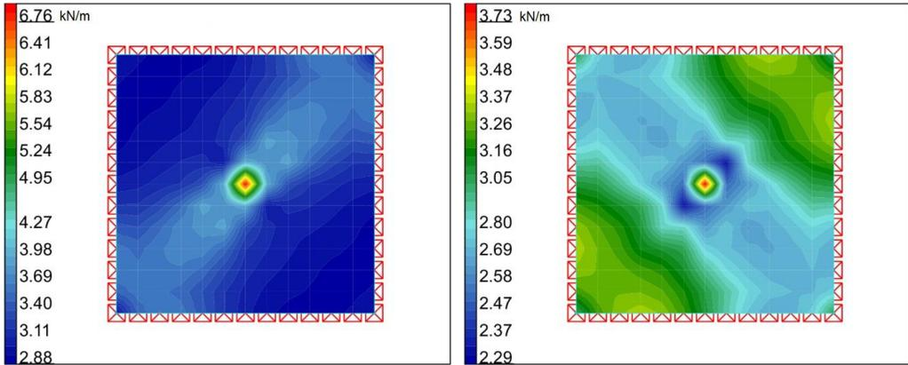
**Figure 6. Membrane forces in warp (left) and weft (right) under 1 kN point load in the center**
