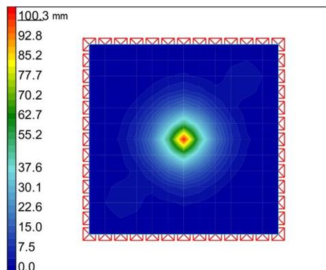
Figure 5. Deflections under  $1 \text{ kN}$  point load positioned in the center
