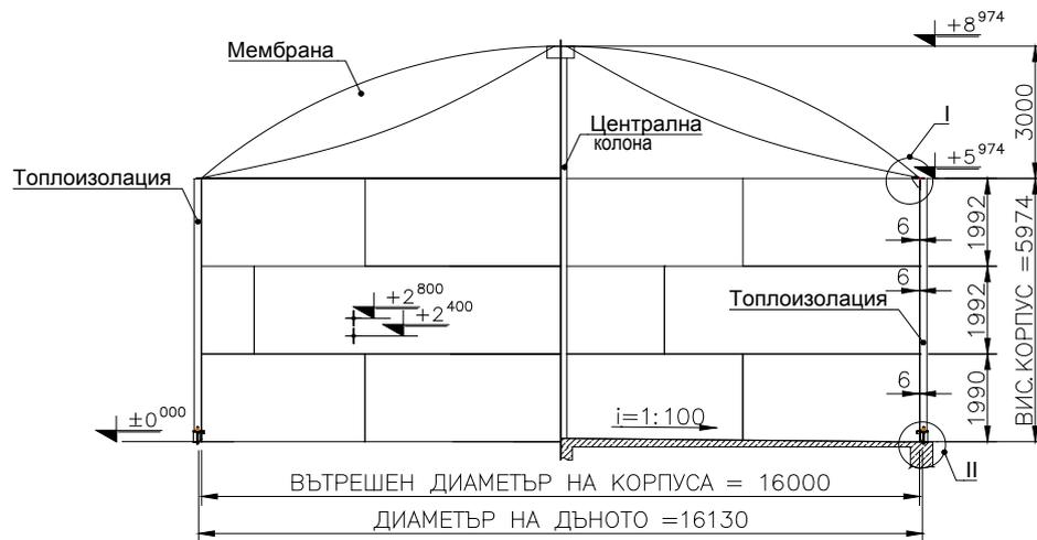
Fig. 6 Gasholder with flexible membrane – general form
