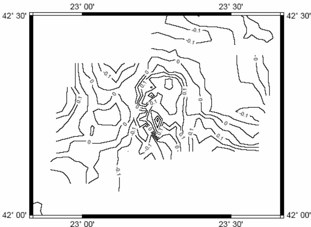
Fig.6. Isolines of the differences between the QBG01 model and the heights from GPS/levelling
