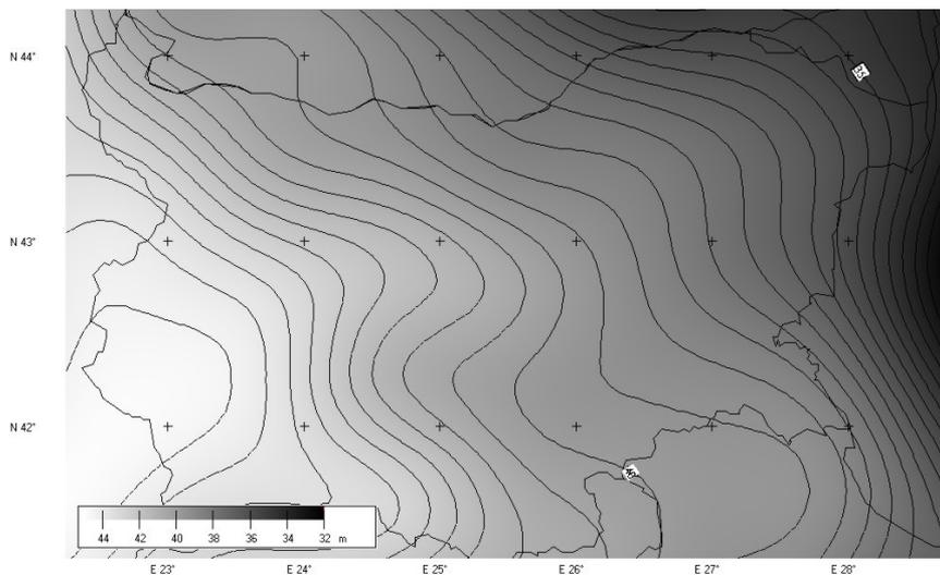
Fig.3. Global model of geoid EGM96 for the studied territory, section of horizontals 0.5 m
