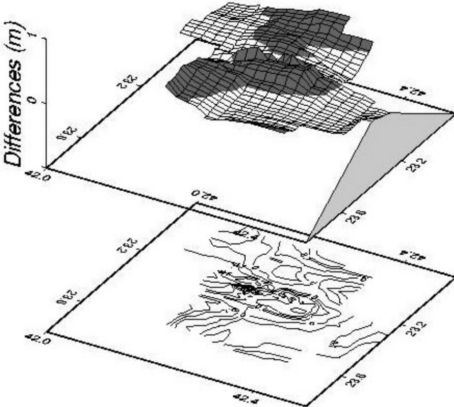
Fig.5. Model of differences between the QBG01 model and the heights from GPS/levelling for a territory restricted within  $\varphi$  42.05°–42.55° and  $\lambda$  22.87°–23.7° after applying the transformation, in [m]
