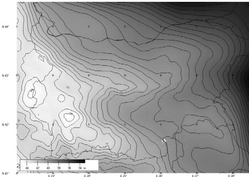
Fig.1. Gravimetric model of the quasigeoid QBG01, section of horizontals 0.5 m
