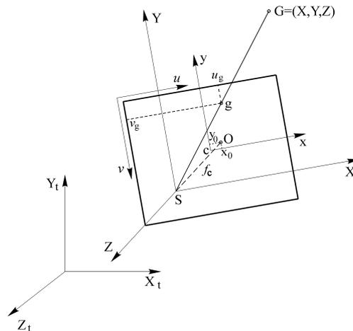
**Figure 2.** Coordinate system for calibration of aerial camera
