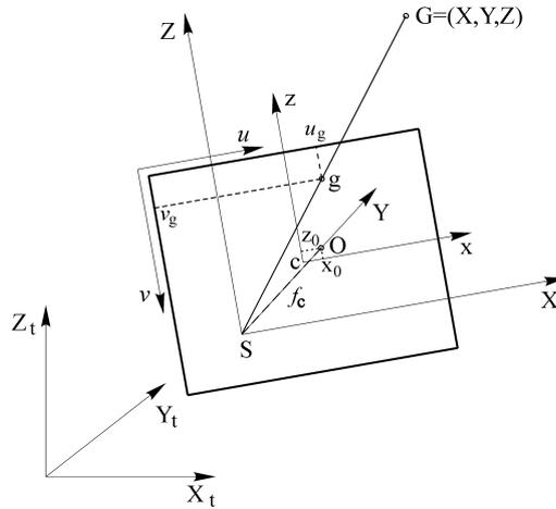
**Figure 3.** Coordinate system for calibration of close-range camera
